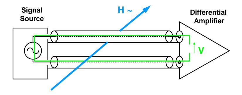
Induced voltage in the loop formed between the coax
