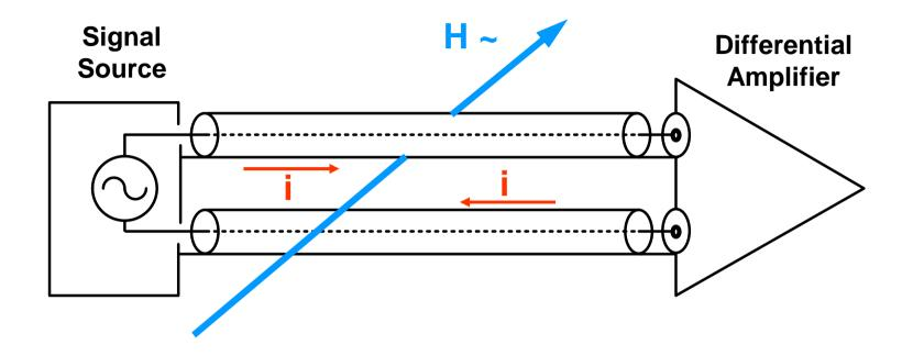
The current i induced in the loop made by the shields are opposed to the flux variation.
