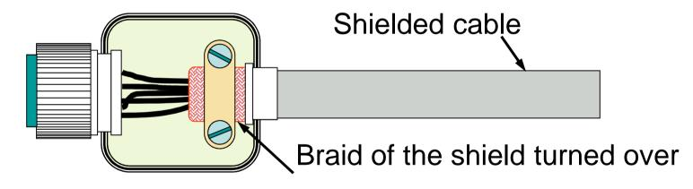
choose connectors which ensure a continuity of the shielding on 360°
