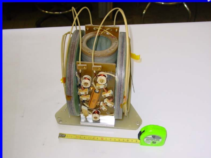
5T (Z) ; 0.5T (X) Without metallic part only use of fiberglass (G11)
