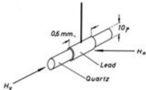
FIG. 1. Schematic diagram of the sample with the directions of the applied field  $H_y$  to be frozen in, and the measuring field  $H_x$ .
