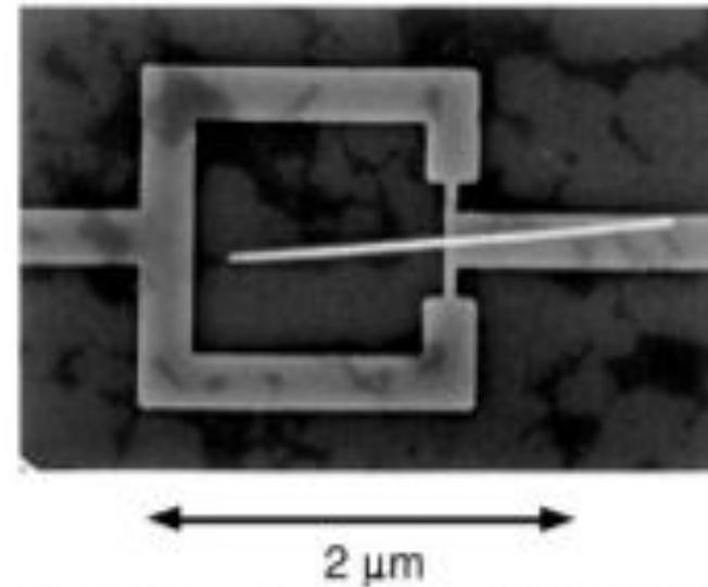
FIG. 1. Scanning electron micrograph (JEOL 6300) of a microbridge de SQUID and a Ni wire of diameter of  $65 \pm 4$  nm.
