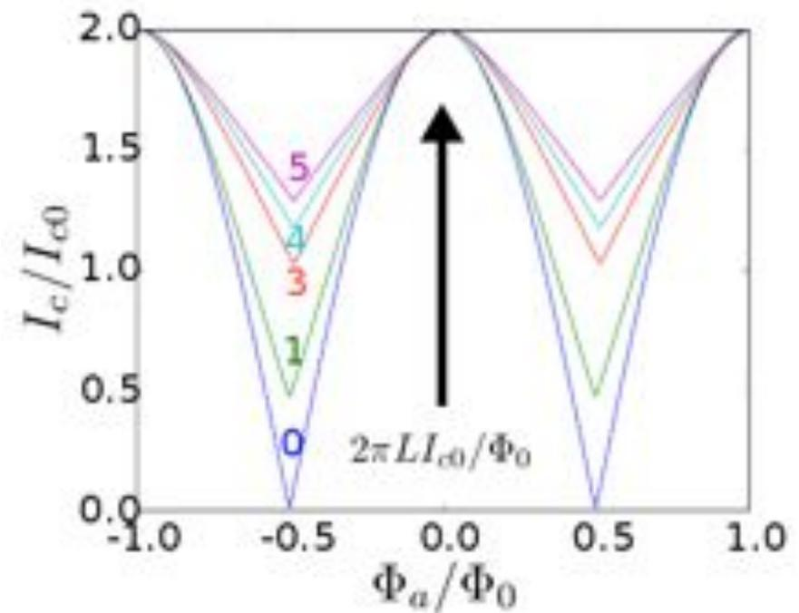
Flux penetrating the SQUID loop modulates the critical current
