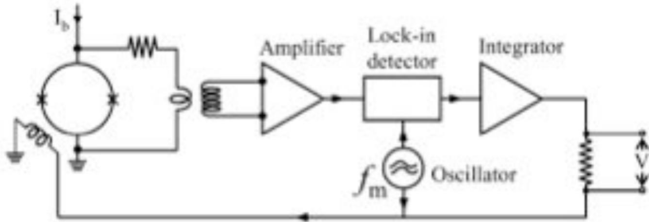
Fig. 4. FLL for operation of a dc SQUID.
