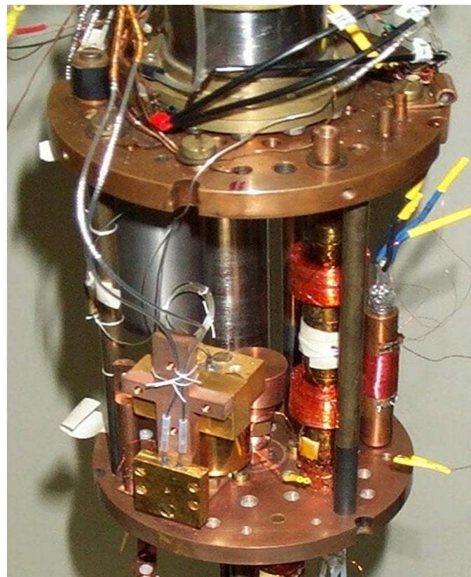
The thermometer stage of the NPL dilution refrigerator below (and isolated through a heat switch from) the mixing chamber, loaded (from left to right) with a PTB melting pressure thermometer, a SRM768 device (behind), a  $^{60}\text{Co}$  nuclear orientation thermometer (at the centre), a CMN thermometer and a rhodium-iron resistance thermometer. The  $\text{PrNi}_5$  nuclear coolant is suspended beneath the plate and is not shown.
